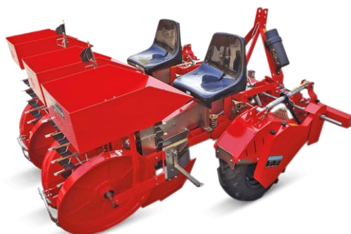
Fig 4: Chechi & Magli Planting Machine, Fox drive model, for bare-root plants (C&M, 2022).
