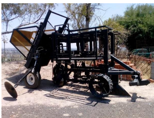
Fig 3: Agave Planting Machine Prototype.
